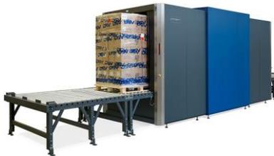
Non-Computed Tomography (Non-CT) Transmission **X-Ray** Constructs **two dimensional X-Ray images** of the cargo item being screened
