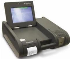
An ETD device analyzes **collected samples** for the presence of **explosive residue**
